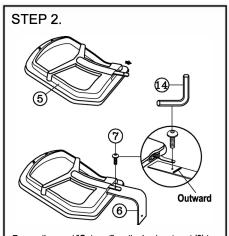
Ensure the word "Outward" on the backrest post (9) is facing outward and the text is the right way up. Please note the backrest post may initially be tight to assimble.
